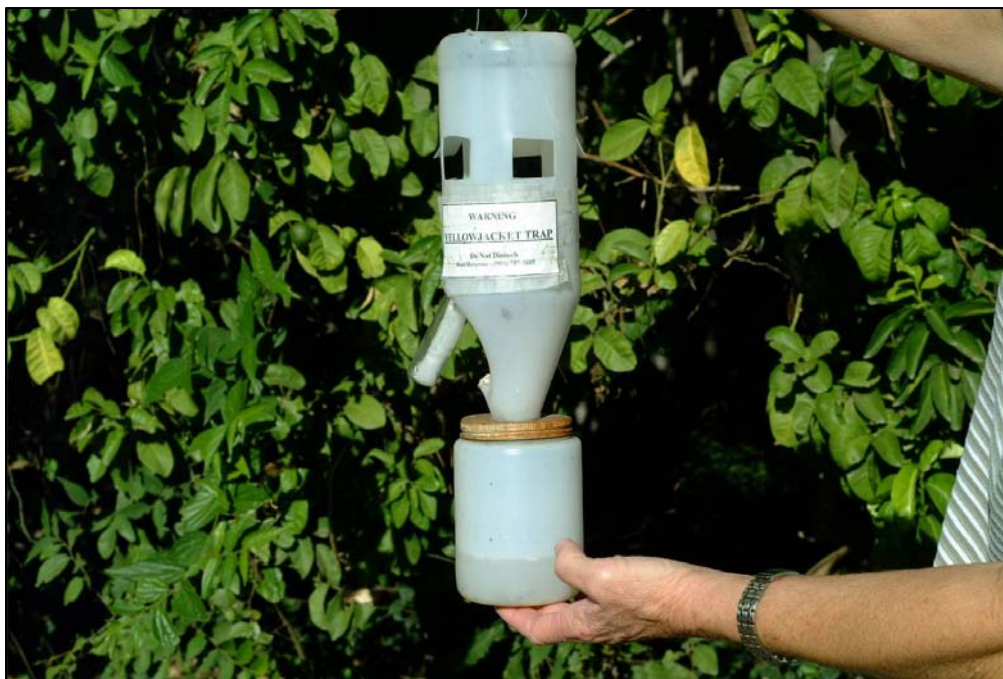
Fig. 2. Two-part UCR yellowjacket bottle trap. Glass vial protruding from right side contains heptyl butyrate dispensed from dental wick, collecting liquid in bottom.
