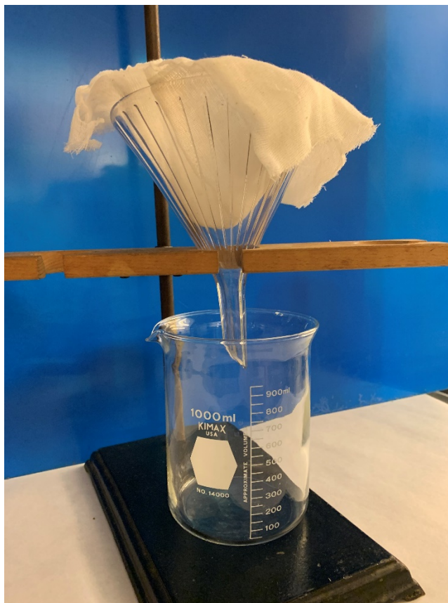
Fig. 22. Extract juices from canned minced chicken and whitefish pet food through cheesecloth.
