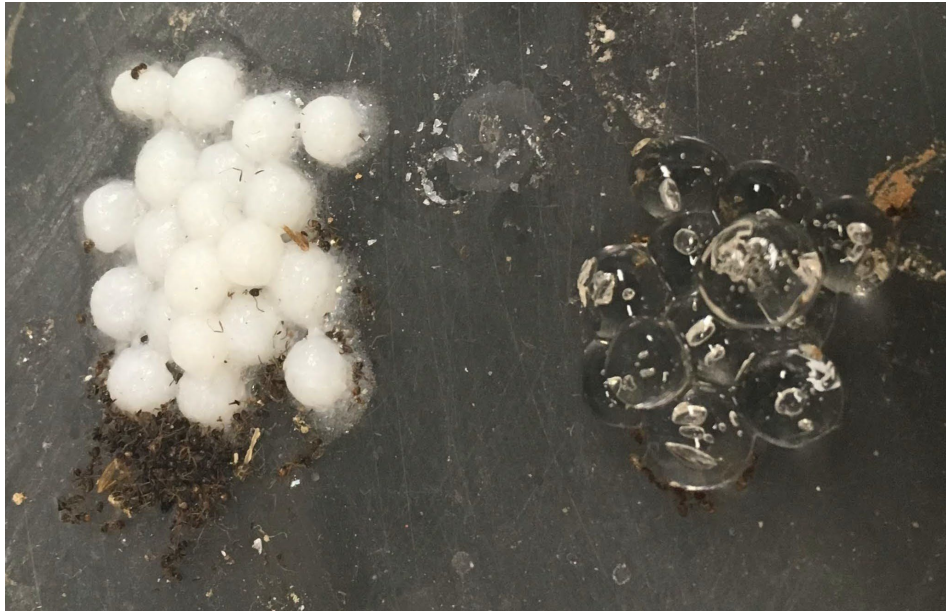
Fig. 5. Rehydration test with the final hydrogel bait. The hydrogel bait beads on the left are completely dried. When enough amount of water is provided, these dry hydrogel beads can be rehydrated (right), becoming palatable to foraging ants once again.
