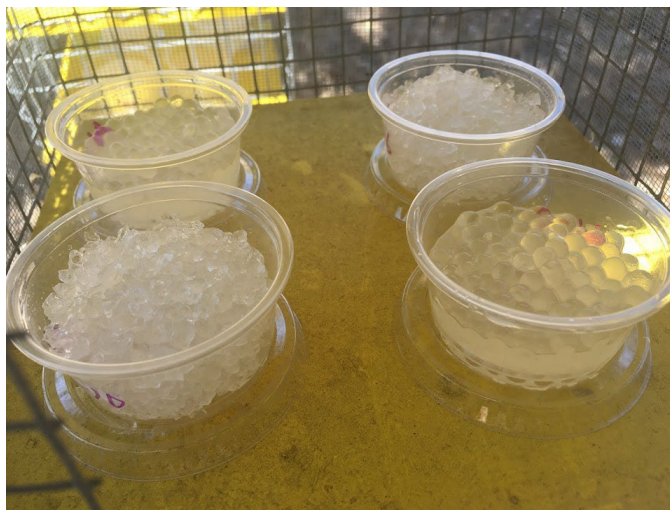
Fig. 23. Gel cups inside of a bait station. From the lower left, clockwise, cups contained PAA, ALG, PAA, and ALG hydrogels. The ALG hydrogels are spherical, and PAA hydrogels have an irregular shape.
